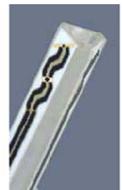
Figure 3.2 Probe Thick-Film Technique
