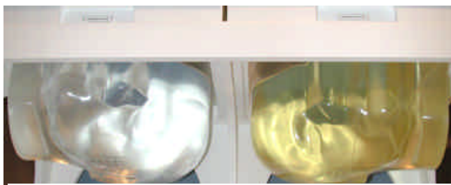
Figure 7.1 Left and Right SAM Phantom shells
