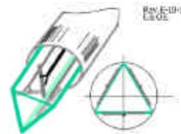
Figure 3.2 Triangular Probe Configuration
