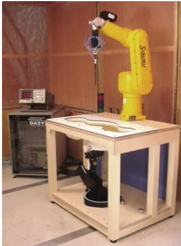
DASY3 SAR Measurement System with SAM phantom
