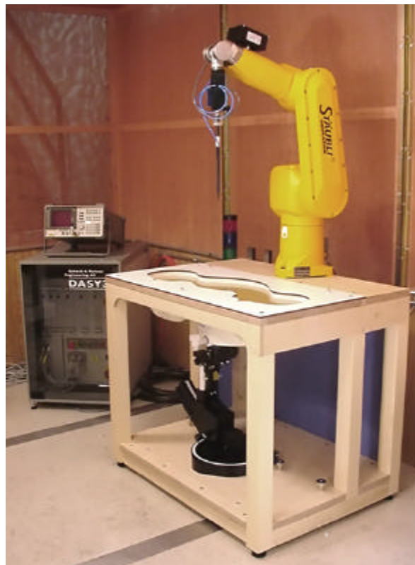
DASY3 SAR Measurement System with SAM phantom
