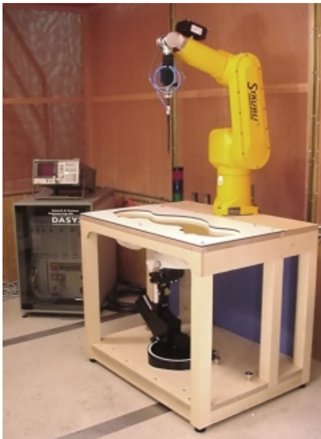
DASY3 SAR Measurement System with SAM phantom
