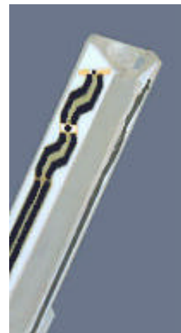
ET3DV6 E-Field Probe
