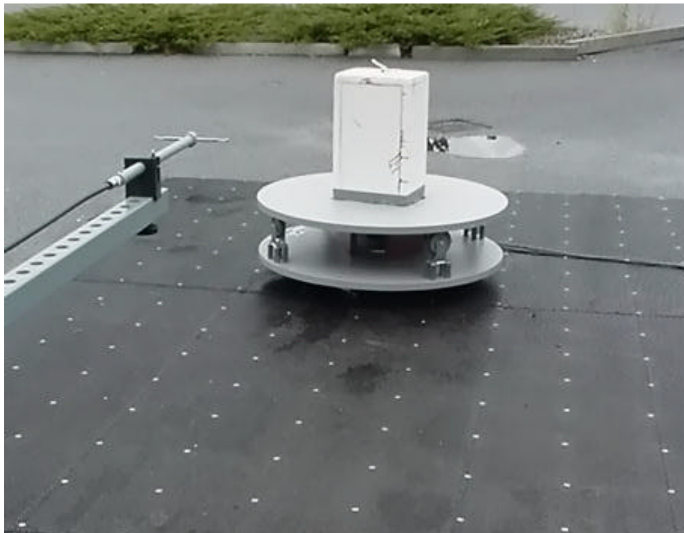
Radiated Measurement Test Setup Photograph
