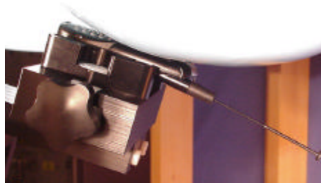
Head SAR Test Setup
