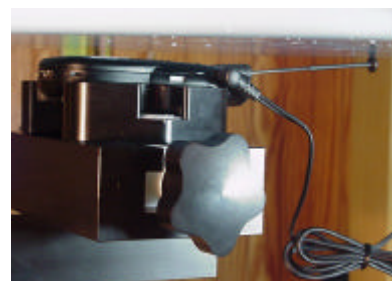
Body SAR Test Setup with 0.5cm spacing
