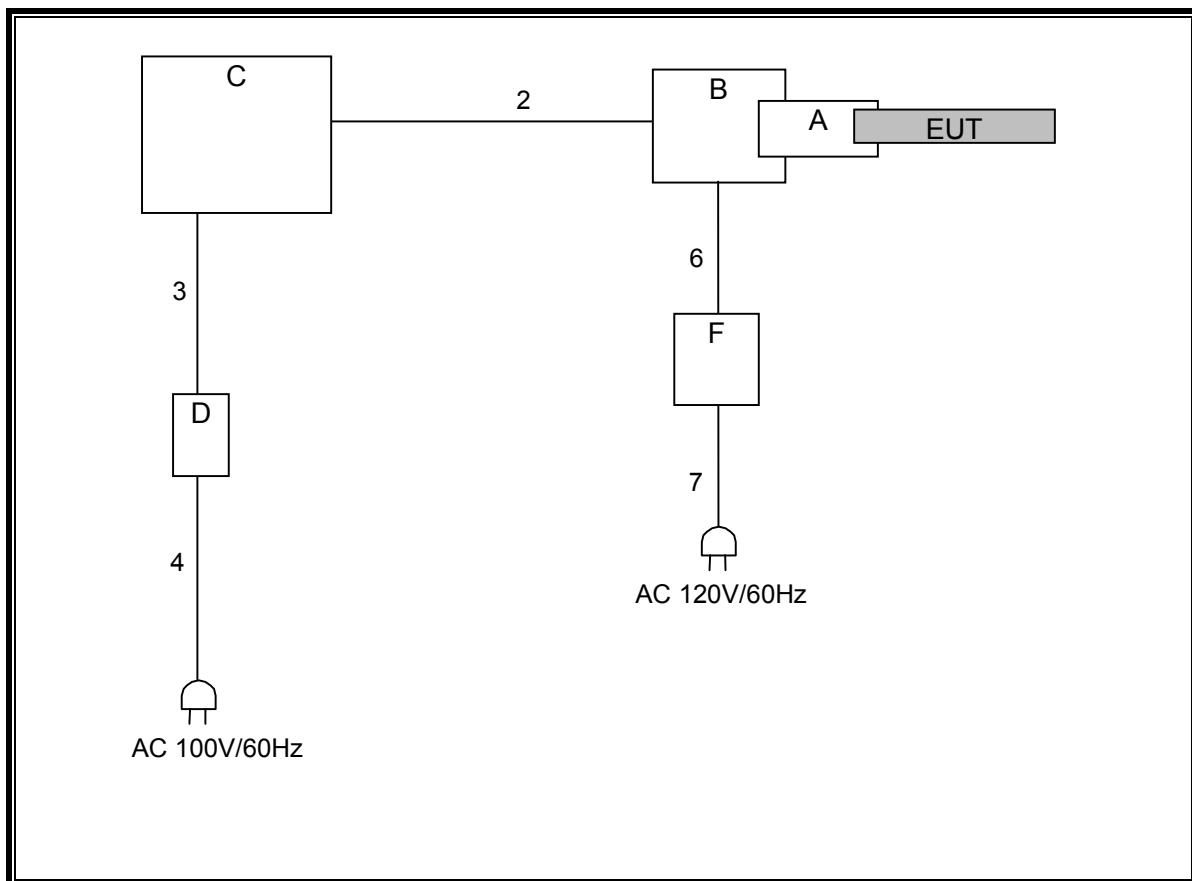
**SETUP DIAGRAM FOR RADIATED EMISSIONS TEST**
