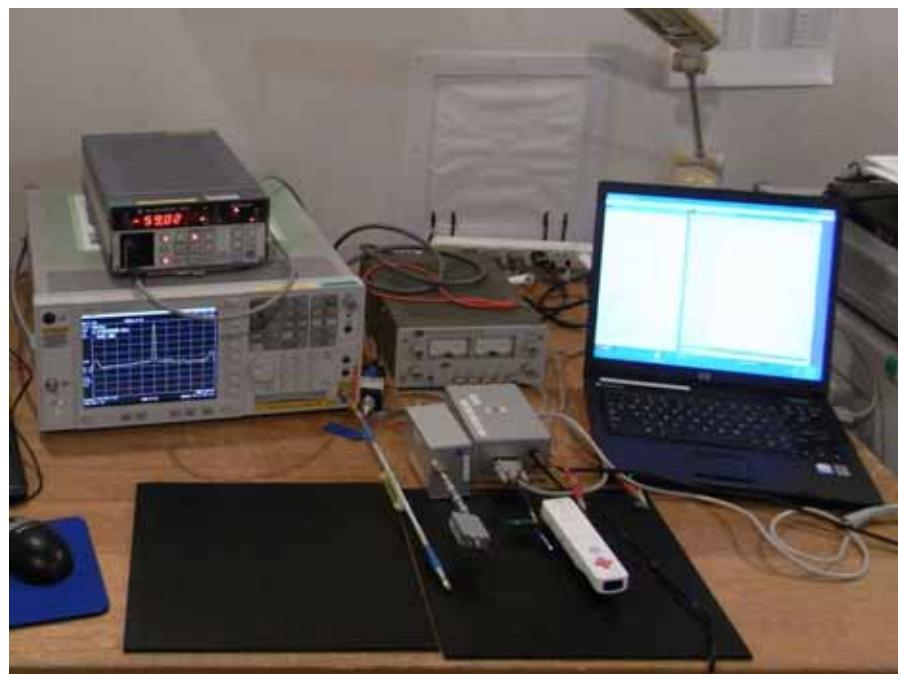
***Transmitter Radiated Spurious Emissions (RF Radiated test)***
