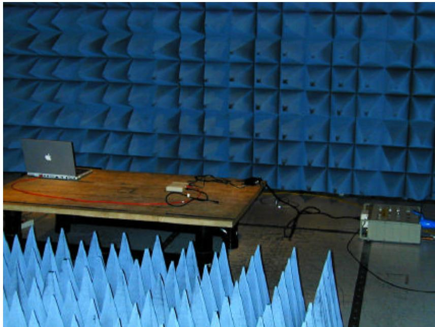
*EQUIPMENT: S75 Satellite Receiver***Section 5. Radiated Emissions****Para. No.: 15.109****Test Performed By:** Daniel Hynes**Date of Test:** May 6, 2002
