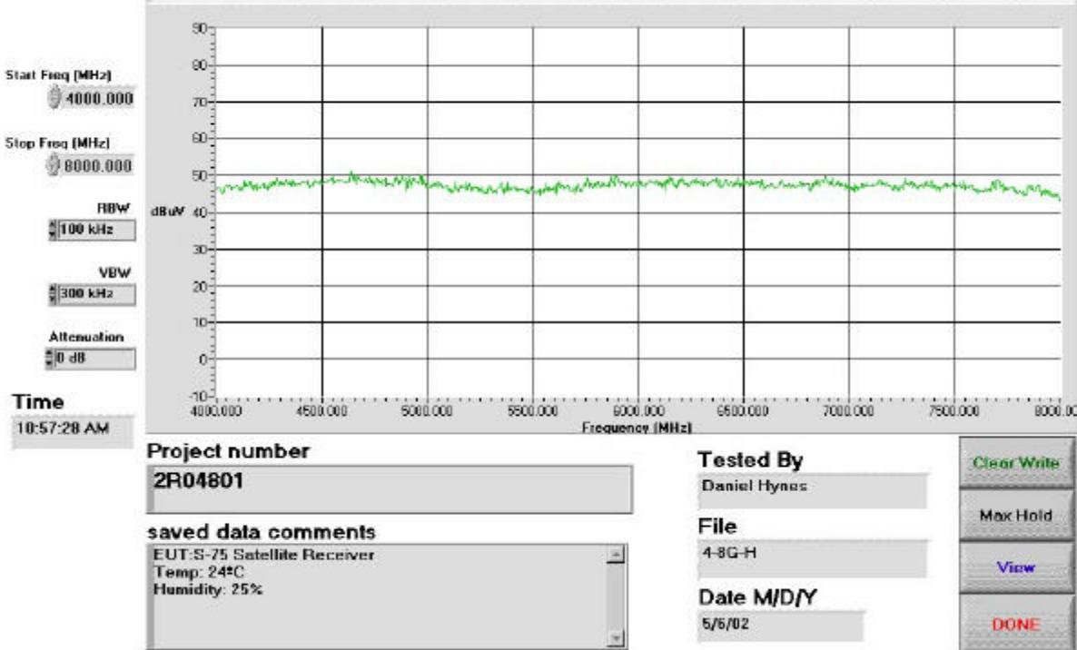
*EQUIPMENT: S75 Satellite Receiver***Radiated Prescan- Vertical**
