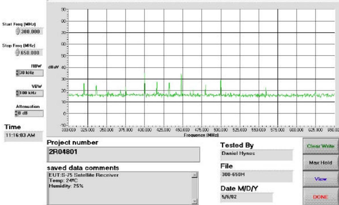
*EQUIPMENT: S75 Satellite Receiver***Radiated Prescan- Vertical**
