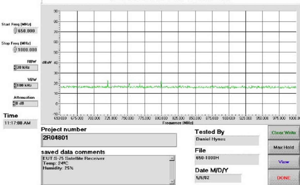
*EQUIPMENT: S75 Satellite Receiver***Radiated Prescan- Vertical**
