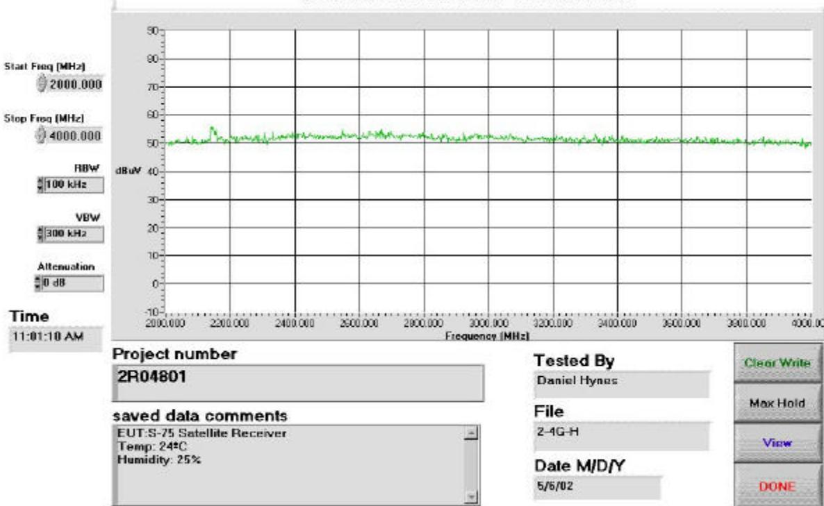
*EQUIPMENT: S75 Satellite Receiver***Radiated Prescan- Vertical**
