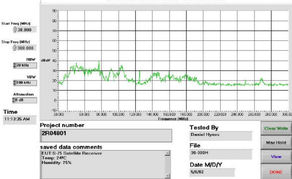
*EQUIPMENT: S75 Satellite Receiver***Radiated Prescan- Vertical**
