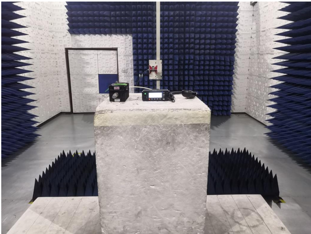
RADIATED EMISSION ABOVE 1G TEST SETUP
