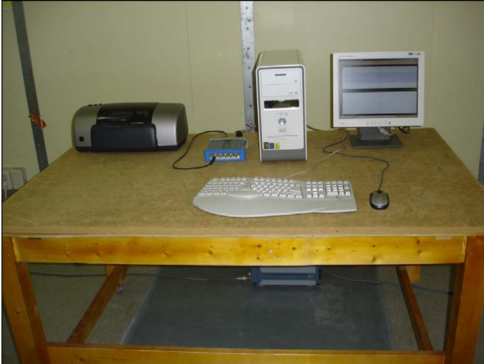
Photograph 1: Setup for Conducted Emissions
