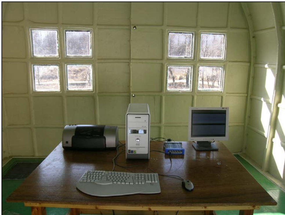
Photograph 2: Setup for Radiated Emissions
