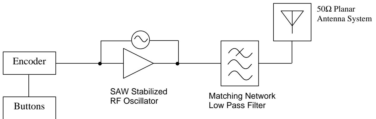
Block Diagram. Same for 418MHz and 433MHz units
