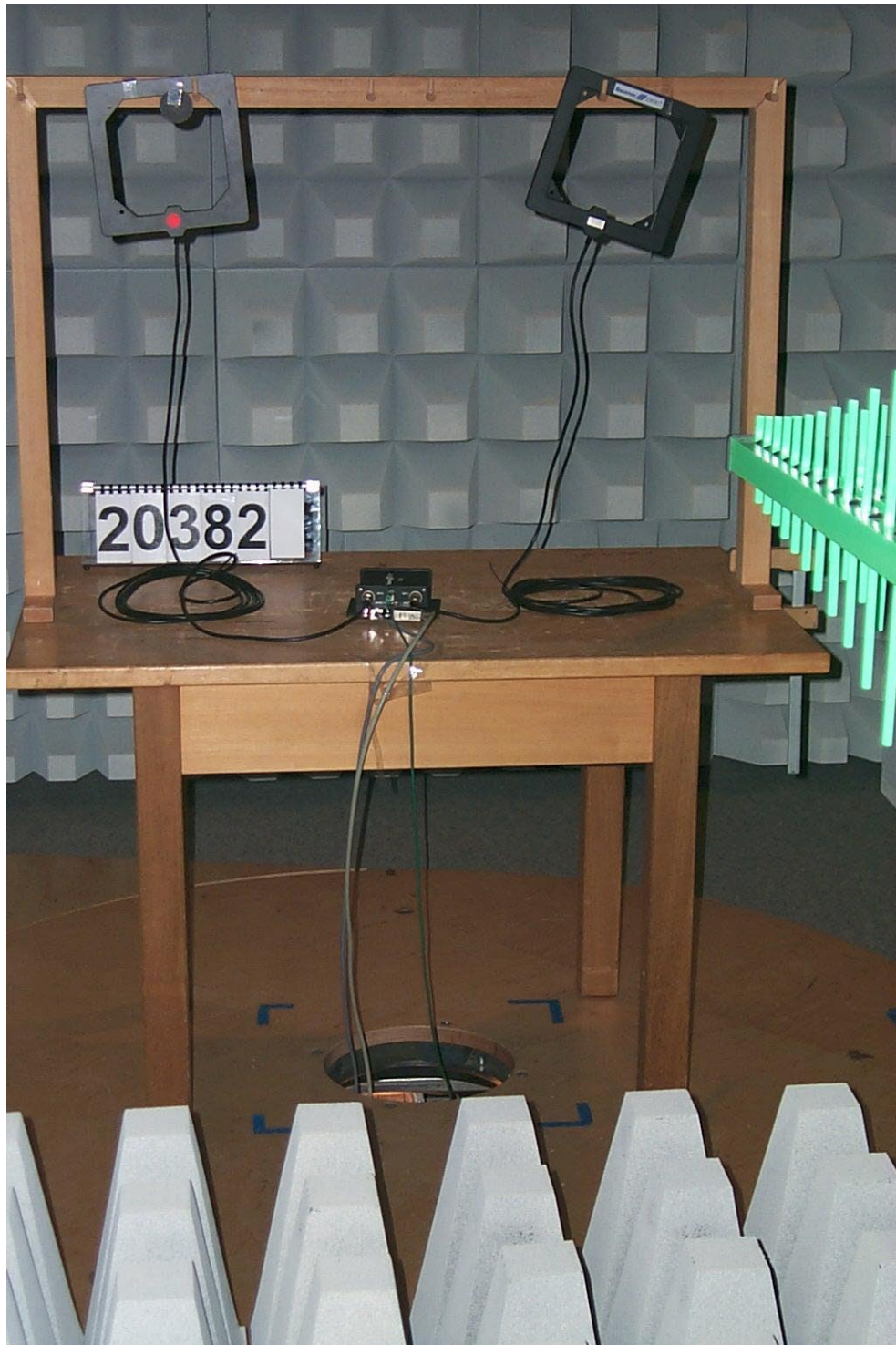
20382_f.jpg OISL 77LA04/2-SER test set-up preliminary emission test (30 to 1000 MHz)
