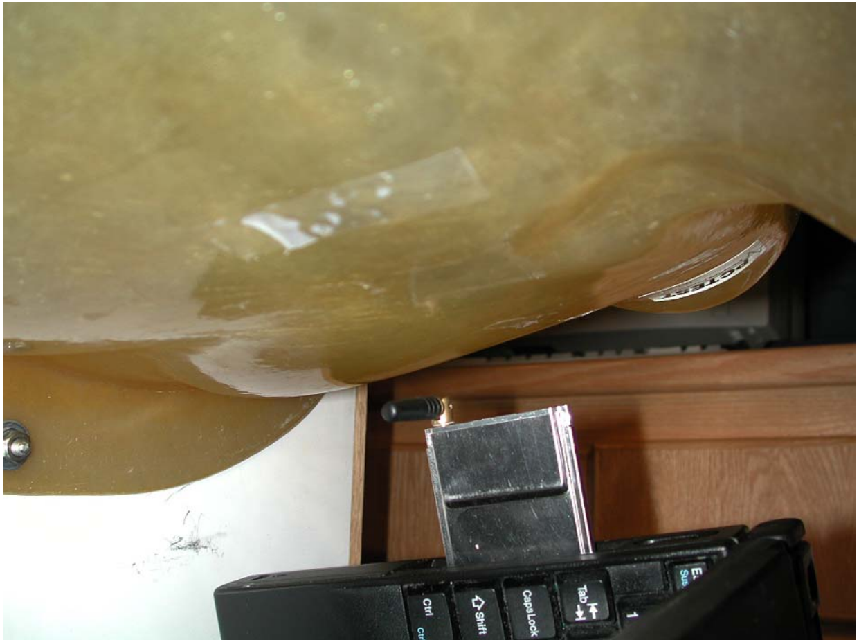
Figure 8. Test Setup of EUT in operating position with the source of significant emissions (antenna) 2.0 cm below the phantom.
