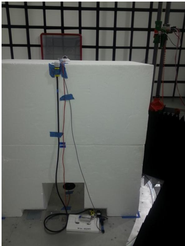
**RADIATED RF MEASUREMENT SETUP FOR PORTABLE CONFIGURATION**
