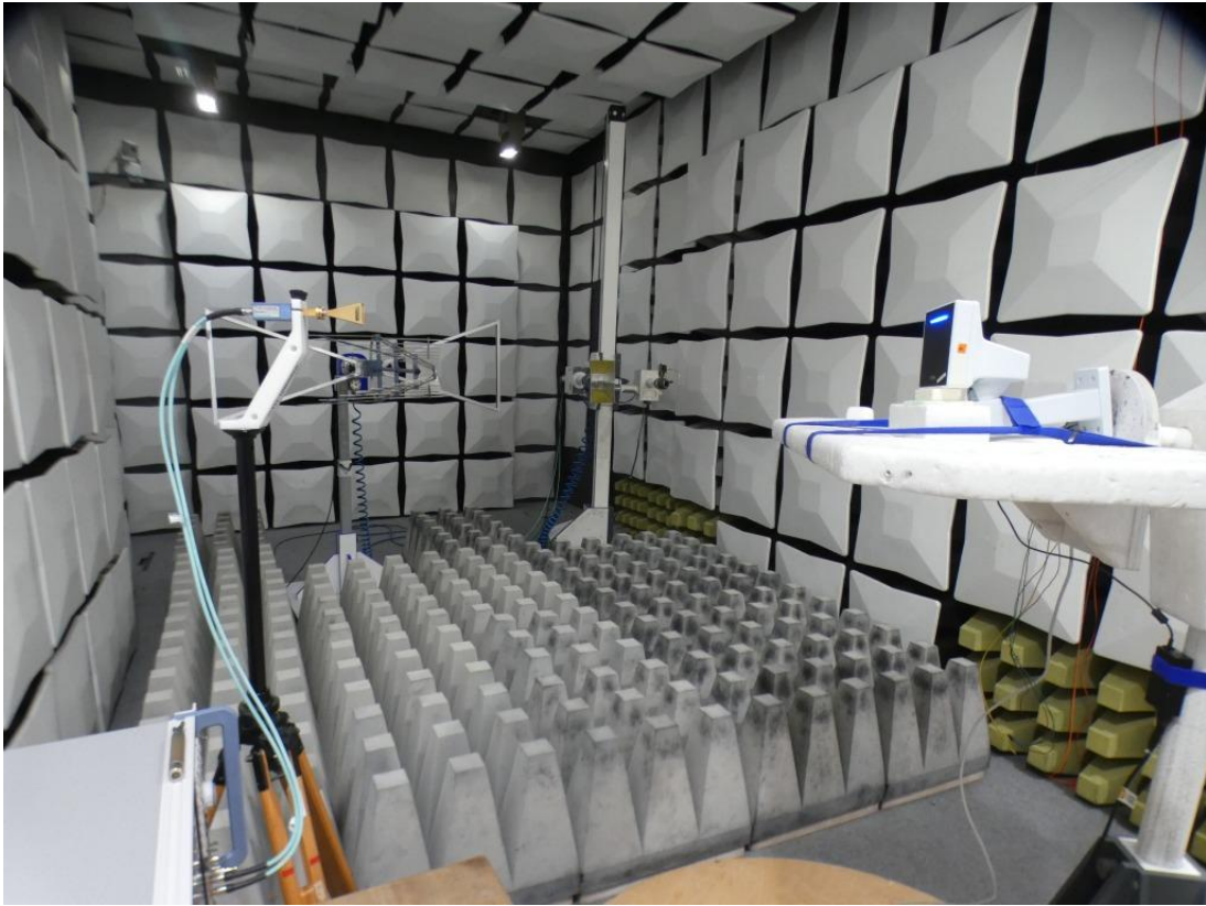
Photo 1: Test setup S01_AA02, for Peak Output Power measurements in the fully anechoic room (FAR)
