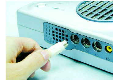
Figure 2-3 Connecting an External Mouse
