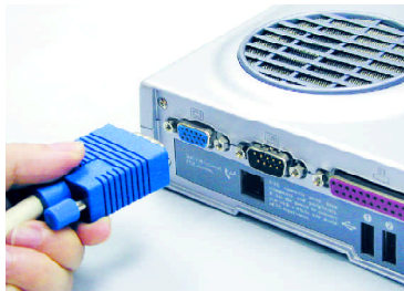
Figure2-4 Connecting an External Monitor
