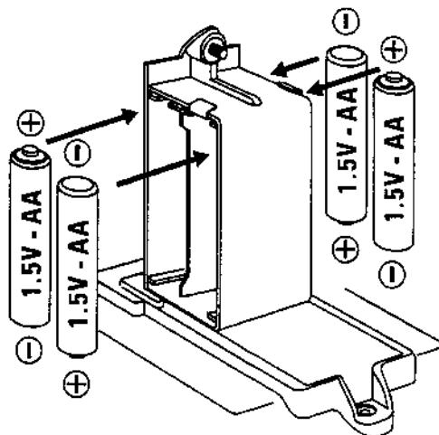
***Battery compartment is located in the bottom of the remote control.***
