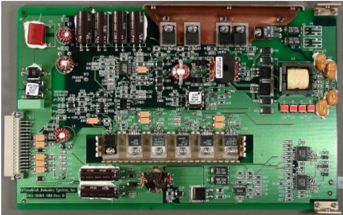
This is the top side of the power supply board.
