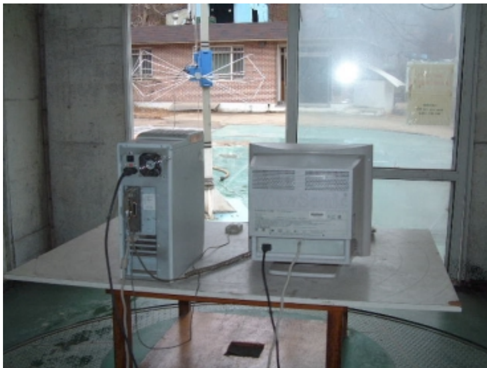
RADIATED EMISSION SETUP PHOTOGRAPH - REAR VIEW ( 30 - 300 MHz )
