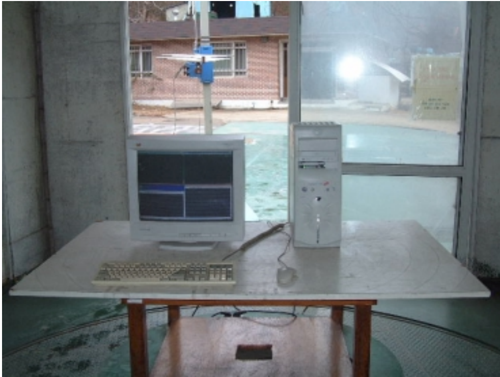
RADIATED EMISSION SETUP PHOTOGRAPH - FRONT VIEW ( 300- 1000 MHz )
