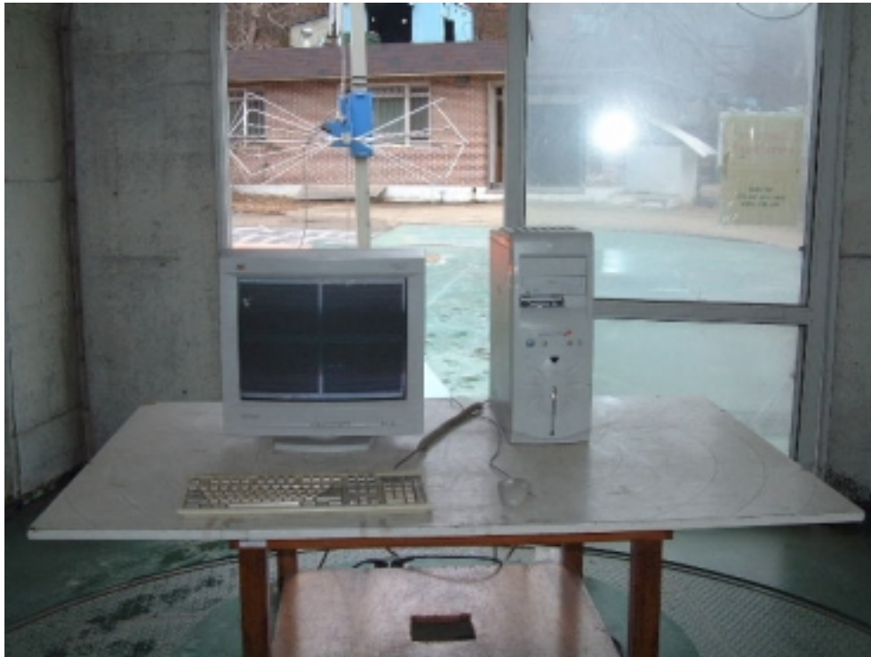
RADIATED EMISSION SETUP PHOTOGRAPH - FRONT VIEW ( 30 - 300 MHz )
