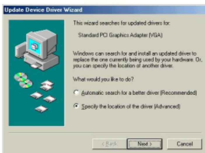
2. From the select Search for a better driver than the one that you are using now. [Recommended] and then check *Specify a location E:\VGA\DRIVER\GeForce2 Series\Win9X*, and then click *Next*. In this case, *E: \ means CD-Rom drive*.
