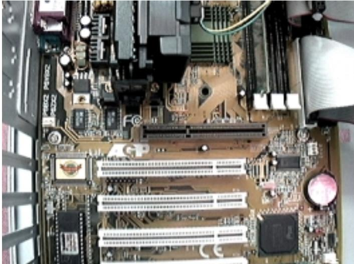
2. Insert your card firmly into the slot. Card should be taken to press it evenly and snugly into its slot. **Do not force!**
