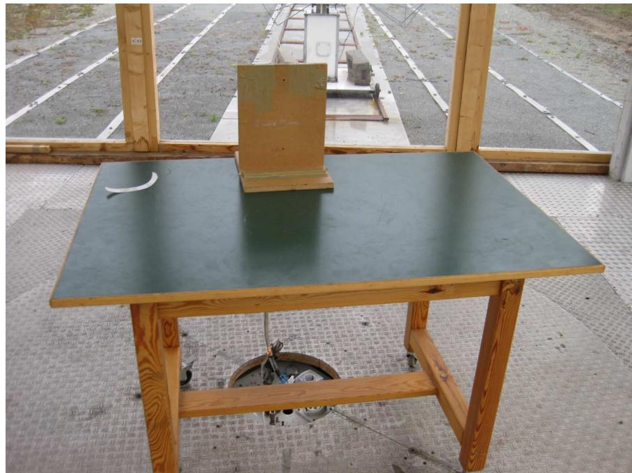
**Test setup for radiated emission measurement
