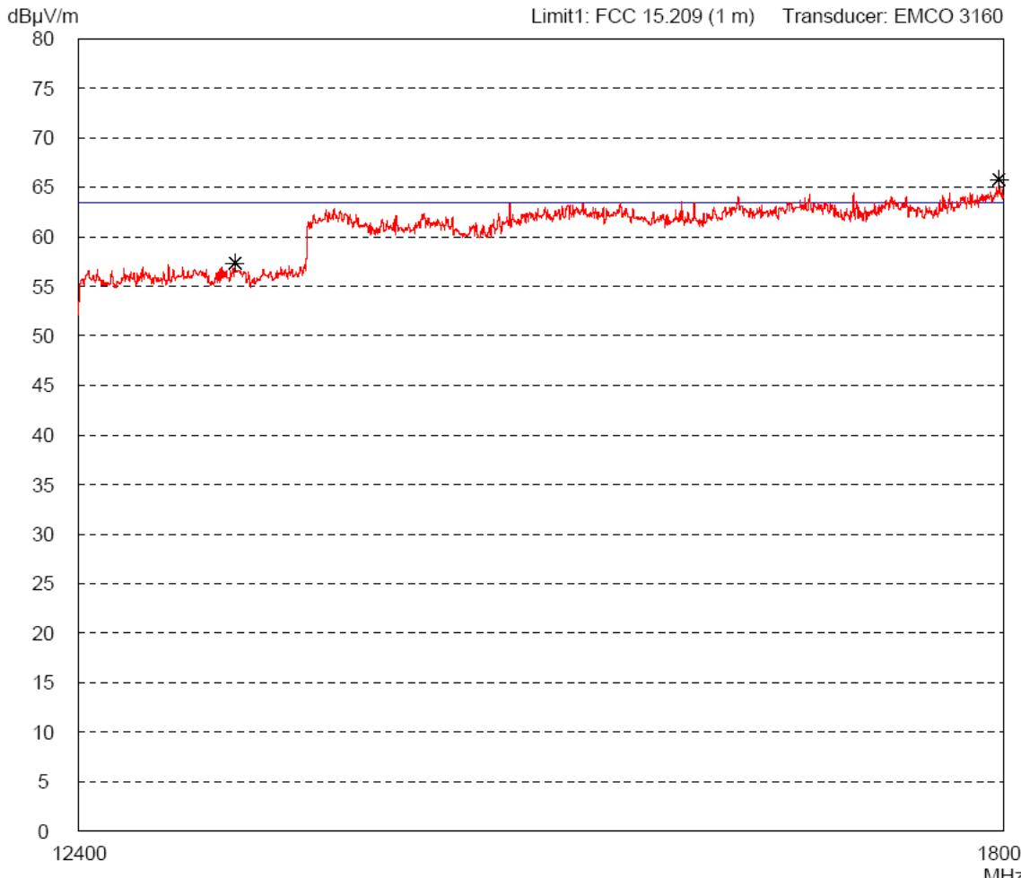
Radiated Emission Test 12.4 GHz - 18 GHz
