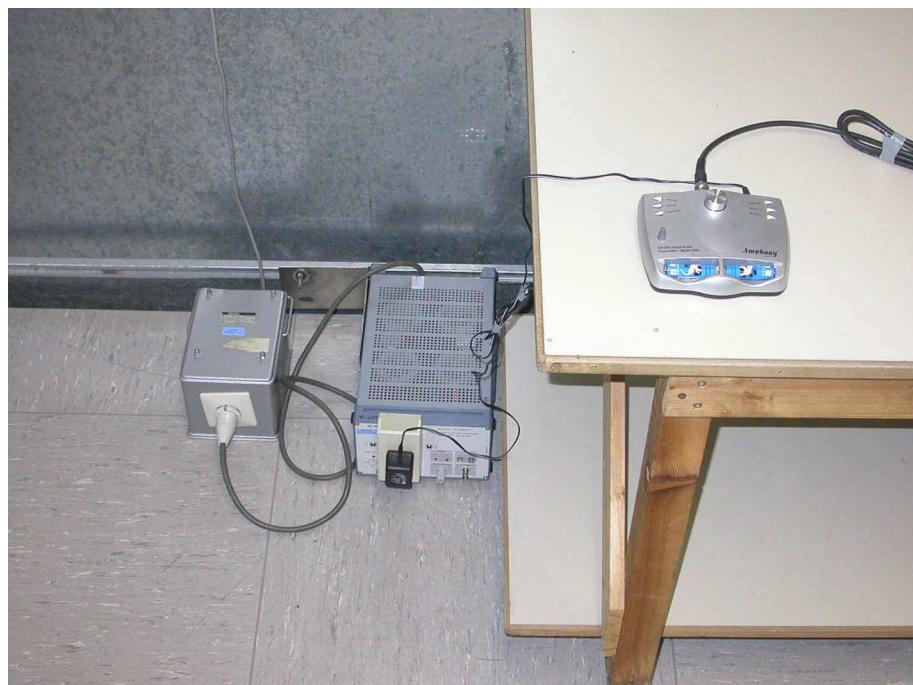
**Test setup for radiated emission measurement
