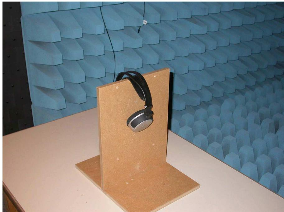
**Test setup for radiated emission measurement
