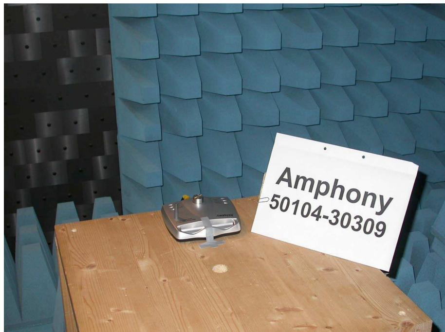
**Test setup for radiated emission measurement
