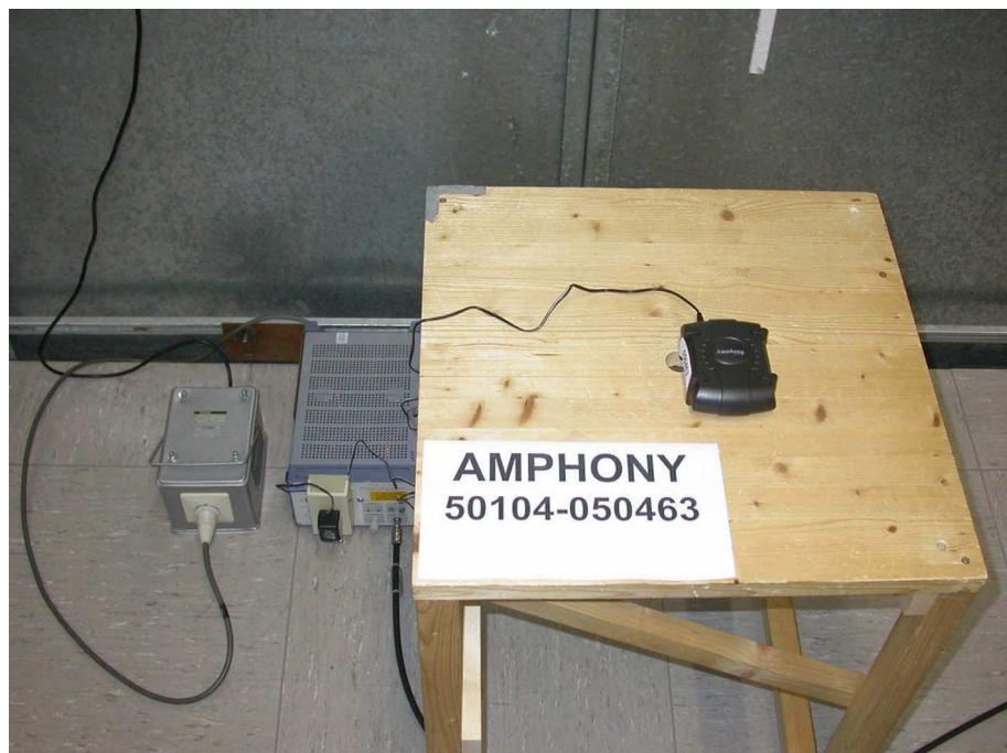
**Test setup for radiated emission measurement
