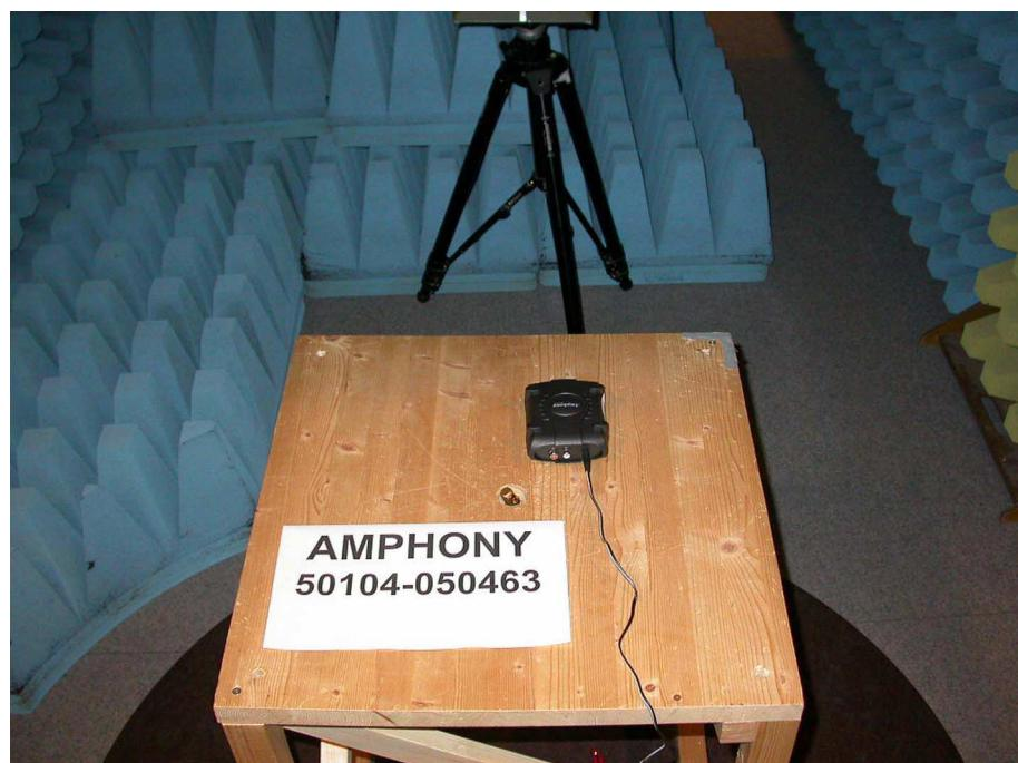
**Test setup for radiated emission measurement
