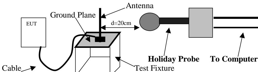
MPE Evaluation was performed using the OET Bulletin 65 or the ANSI/IEEE C95.3, "IEEE Recommended Practice for the Measurement of Potentially Hazardous Electromagnetic Fields - RF and Microwave" test procedure, for mobile devices.
