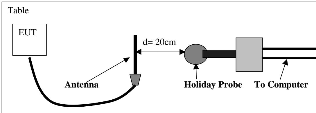
MPE Evaluation was performed using the OET Bulletin 65 or the ANSI/IEEE C95.3, "IEEE Recommended Practice for the Measurement of Potentially Hazardous Electromagnetic Fields - RF and Microwave" test procedure, for mobile devices.
