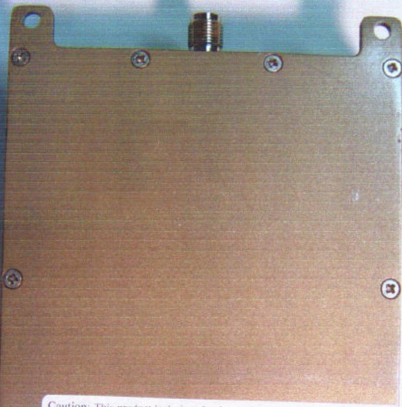
Caution: This product is designed to be used with an external antenna with maximum of 5dBd or 3dB or less. The use of an antenna of higher gain is strictly prohibited and violates FCC regulations.
