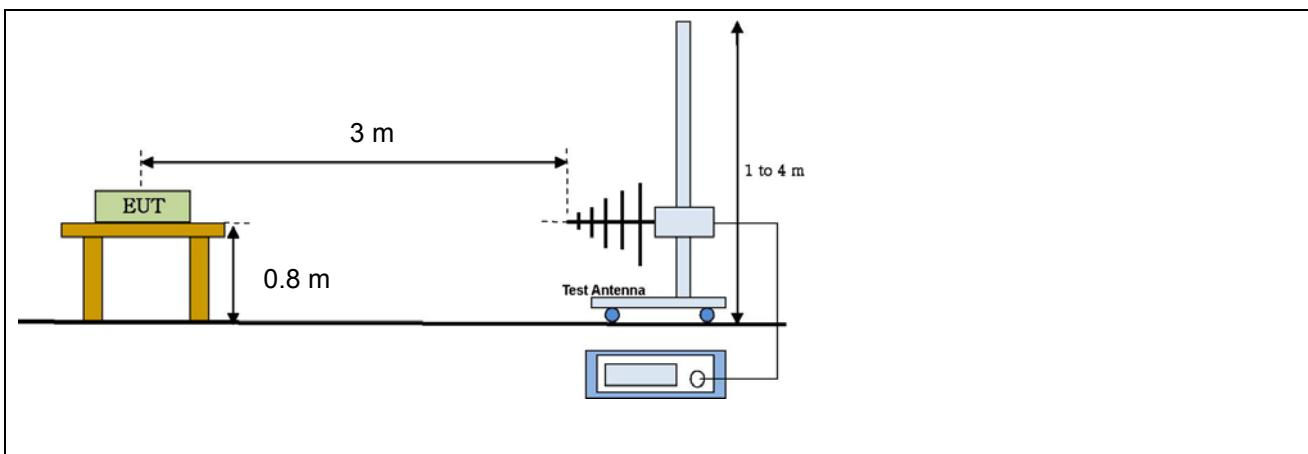
Radiated emission setup, Above 1 GHz
