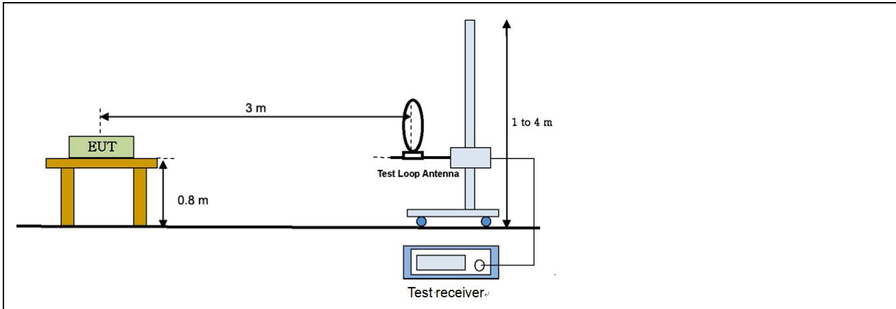
Radiated emission setup, Below 1 000 MHz
