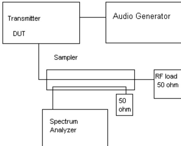
Method of Measuring Conducted Spurious Emissions
