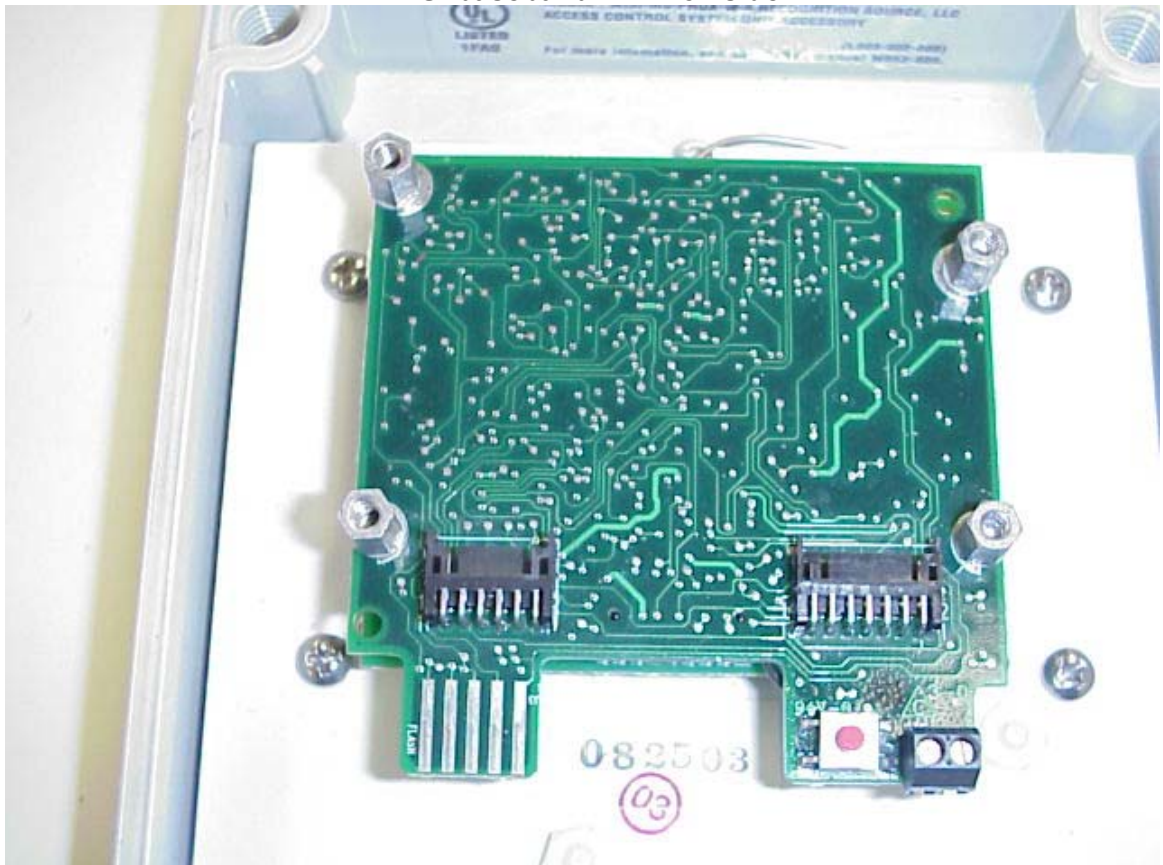
WISI baseband PCB foil side
