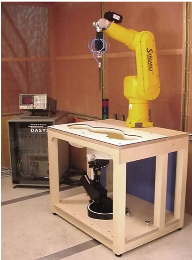
DASY3 SAR Measurement System with SAM Phantom
