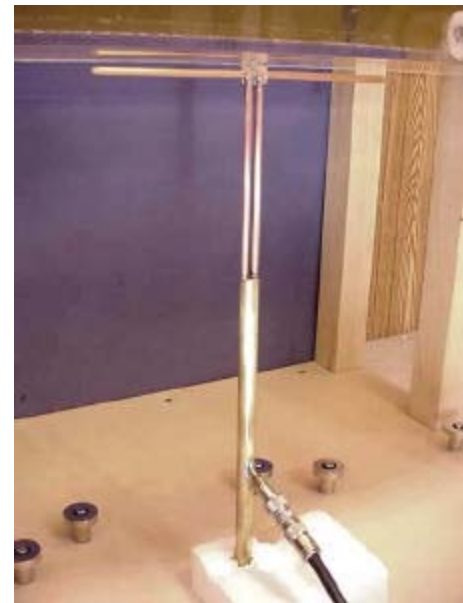
450MHz System Check Setup
