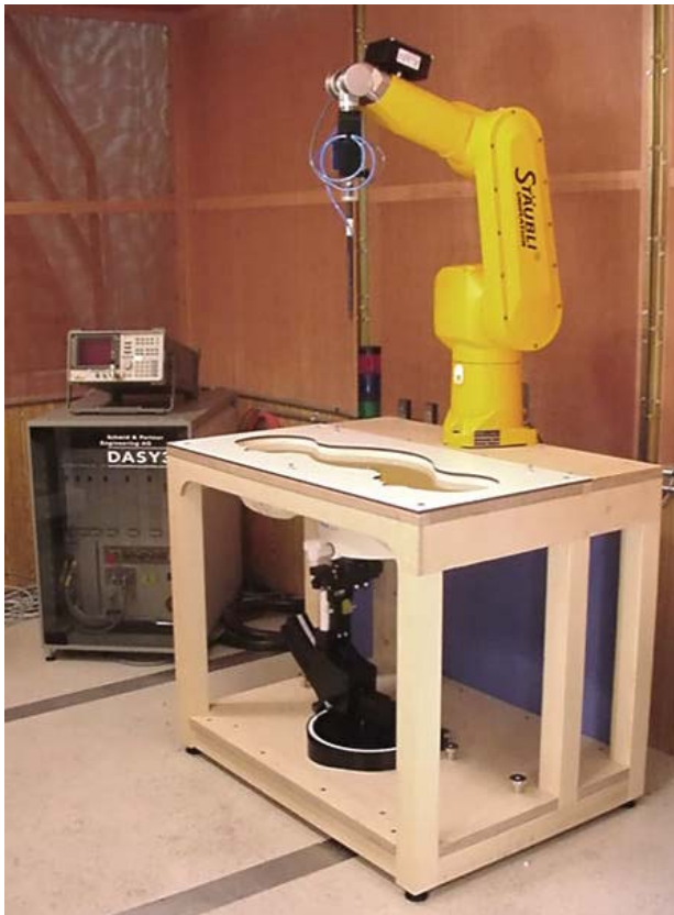
DASY3 SAR Measurement System with SAM Phantom
