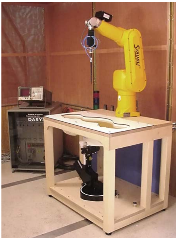
DASY3 SAR Measurement System with SAM Phantom
