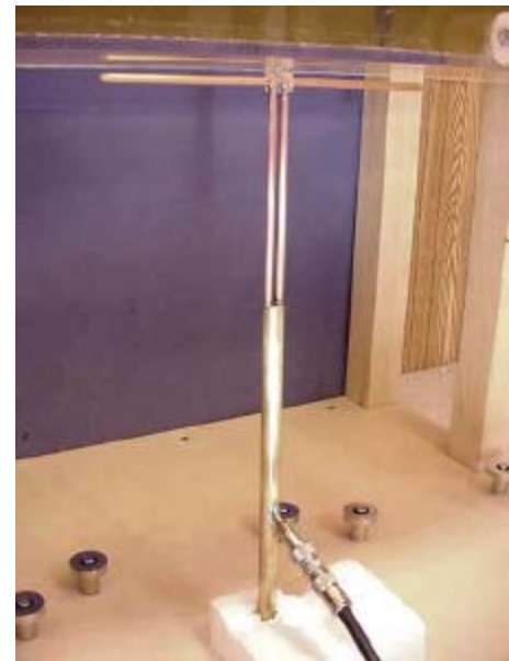
450MHz Dipole Validation Setup
