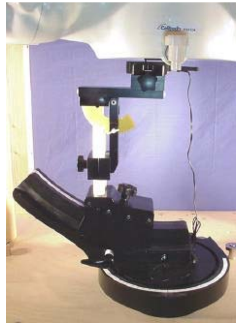
Body-worn SAR Test Setup
