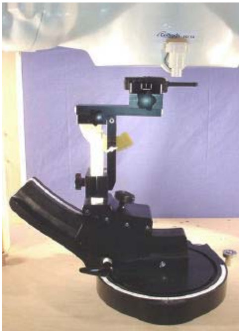
Face-held SAR Test Setup
