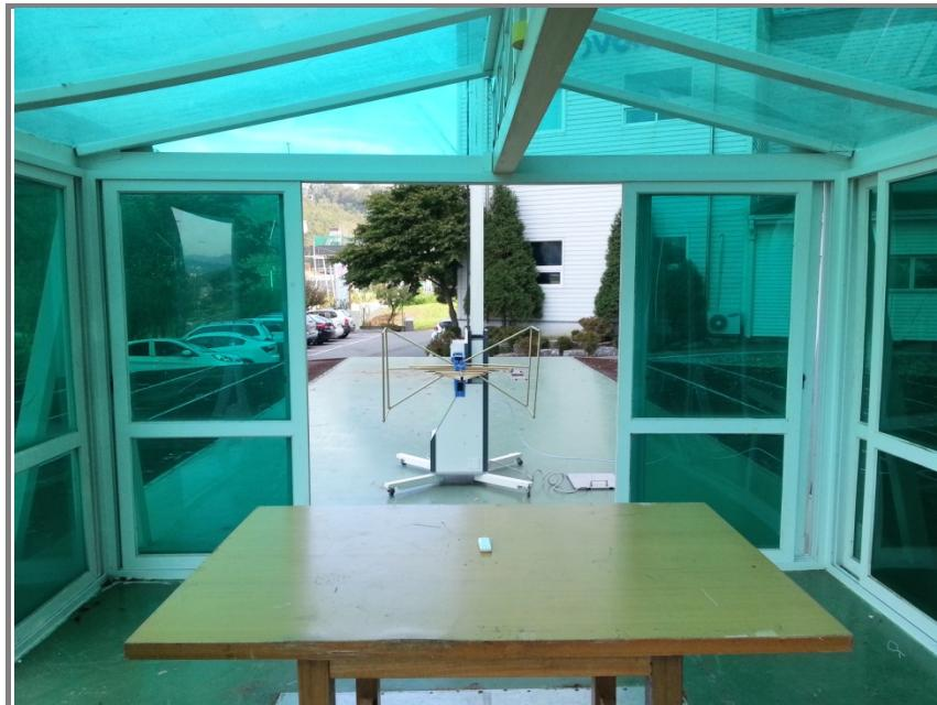
**Photo of radiated spurious emission at above 1 000 MHz**
