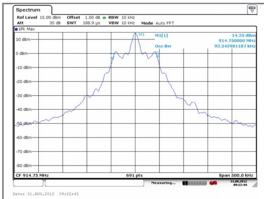
**C. High channel (927.25 MHz) – 20 dB bandwidth & 99 % bandwidth**
