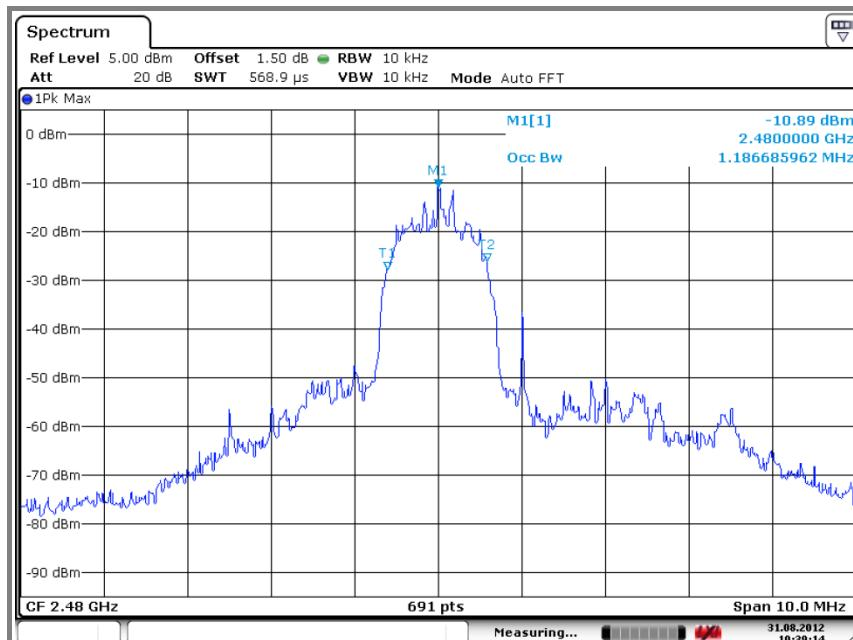
**8. Maximum peak output power measurement****8.1. Test setup.**
