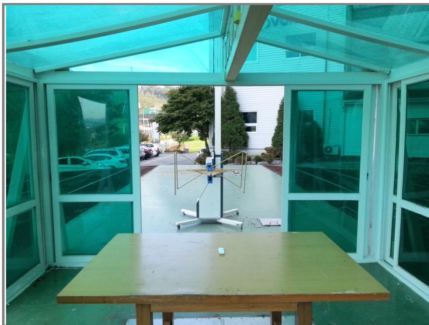
**Photo of radiated spurious emission at above 1 000 MHz**
