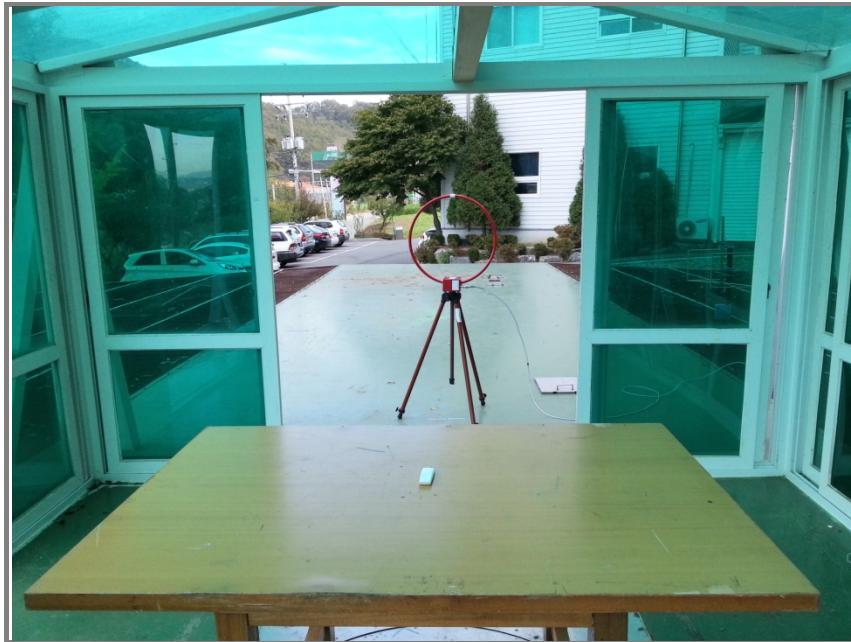
**Photo of radiated spurious emission at 30 MHz ~ 1 000 MHz**
