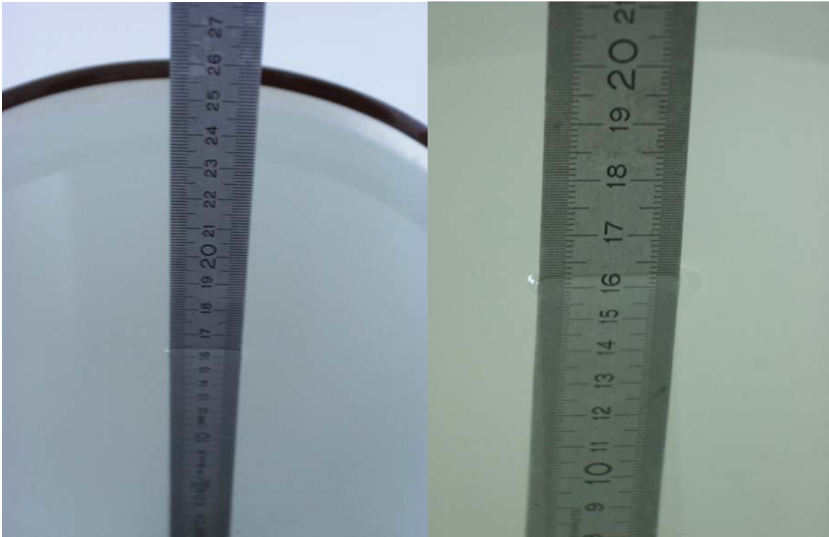
Fig. 21: Liquid depth for PCS 1900 Head and Body measurements.
