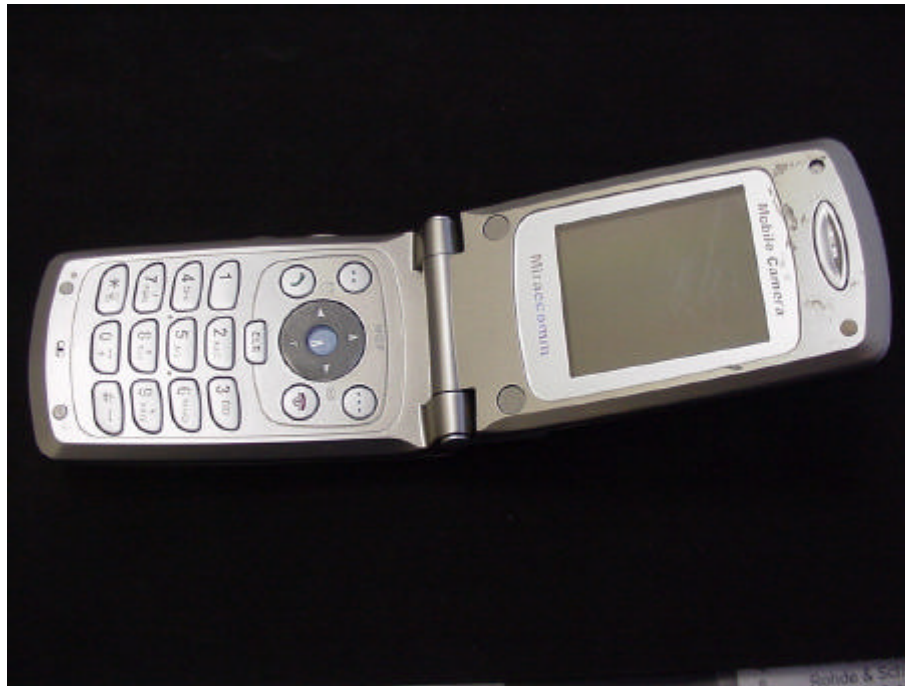
Picture 3 : EUT for radiated tests (front side)
