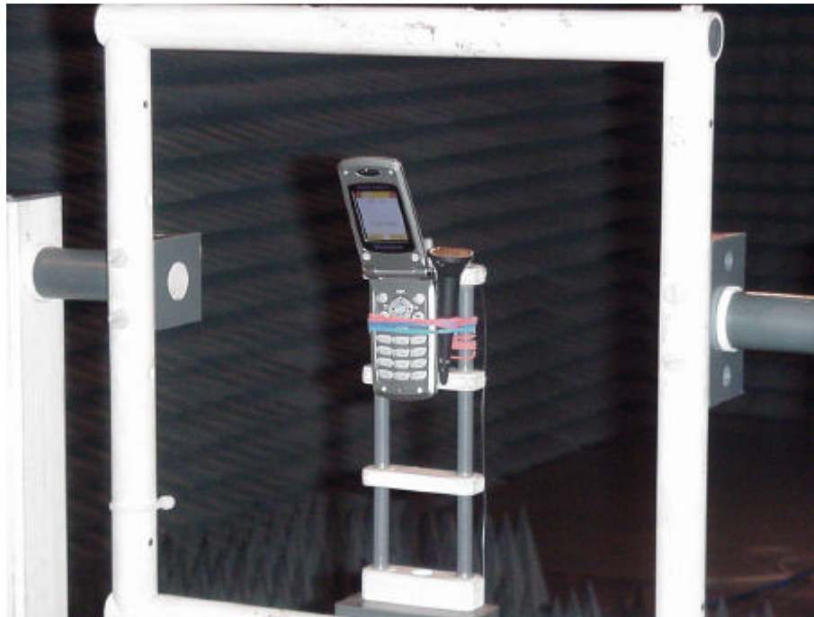
Picture 5 : Test setup for radiated measurements in anechoic chamber
