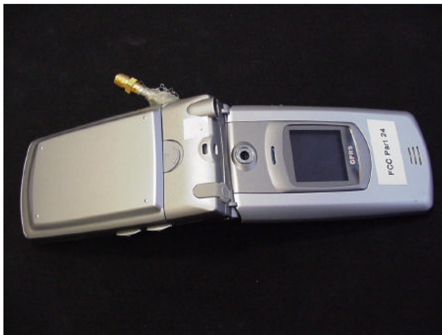
Picture 2 : EUT for conducted tests with temporary antenna connector (front side)
