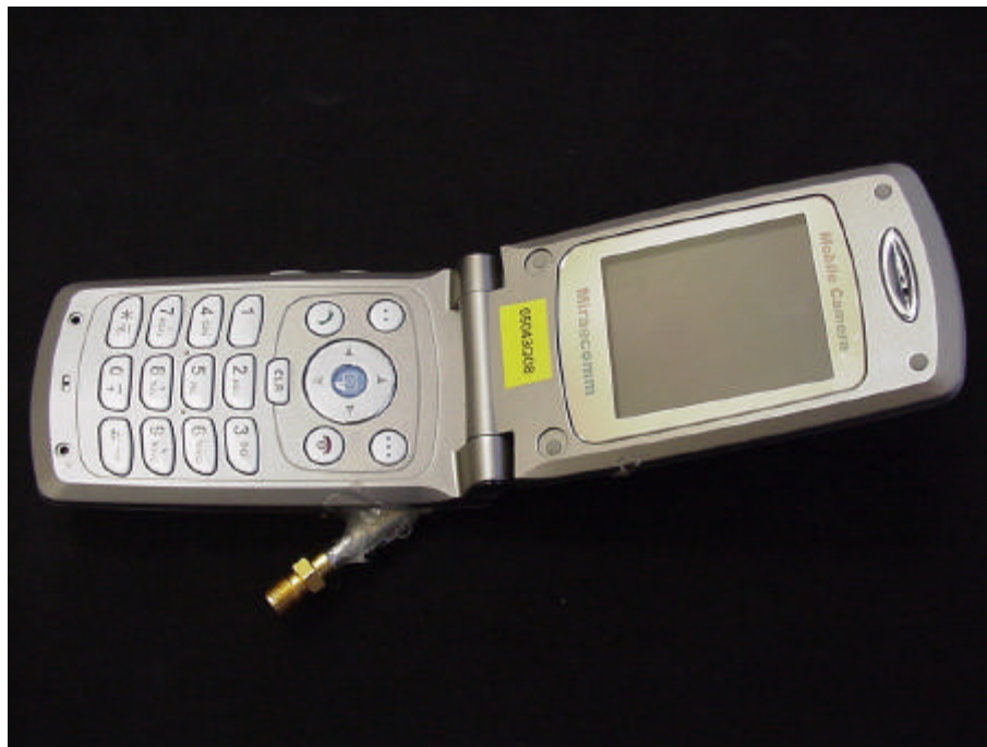
Picture 1 : EUT for conducted tests with temporary antenna connector (front side)
