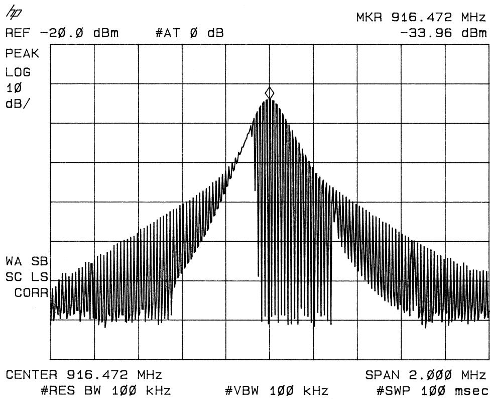
The field strength measurements were taken using an HP8596E spectrum analyzer, an EMCO 3121C dipole set, an EMCO 3115 double ridge guide horn and an Avantek UJ210 preamp. The device was scanned in both transmit and receive modes from 30MHz. to 10GHz. and all emissions were noted. In this case, the only emissions detected were those harmonically related to the fundamental transmit frequency.
