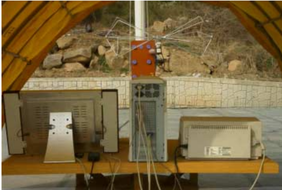
Photograph 1 : Setup for radiated Emissions
