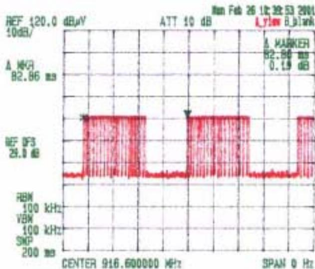
$$T_{on} = 18 \times 1.6 \text{ ms} = 28.8 \text{ ms}$$
