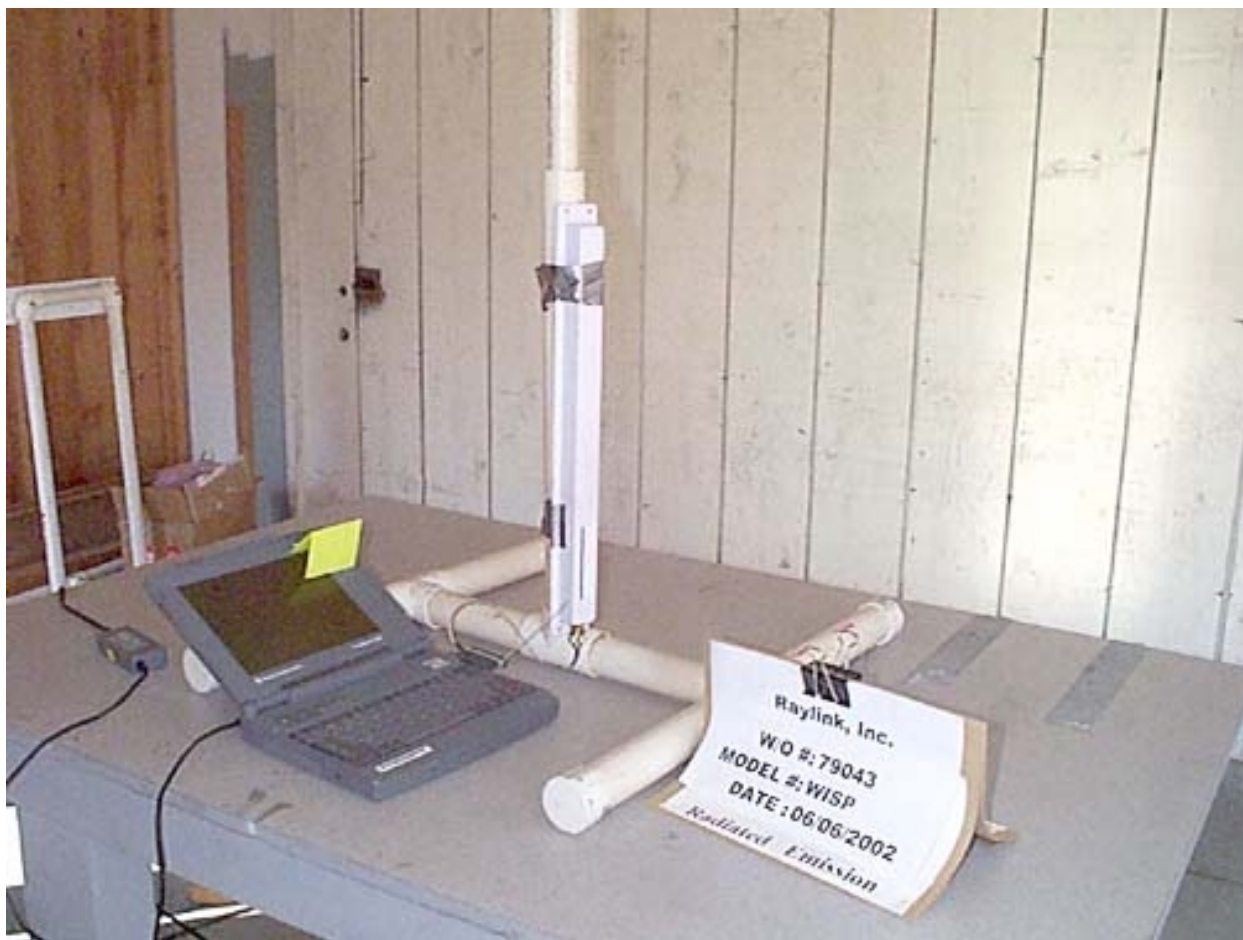
OATS Test Setup - Front View - Biconilog Antenna - Mode A
