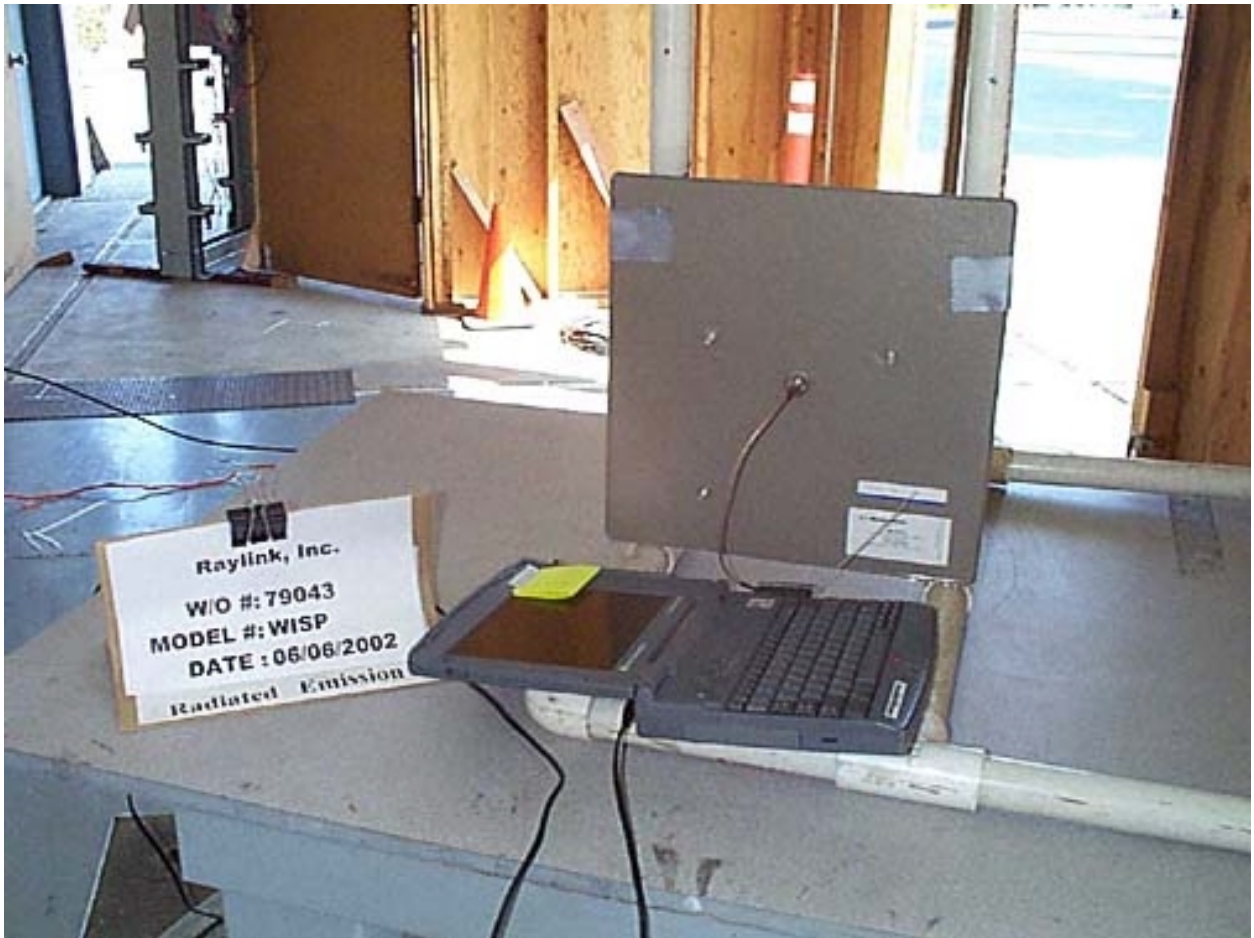
OATS Test Setup - Front View - Biconilog Antenna - Mode B
