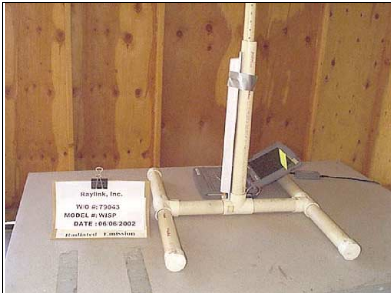
OATS Test Setup - Back View - Biconilog Antenna - Mode A
