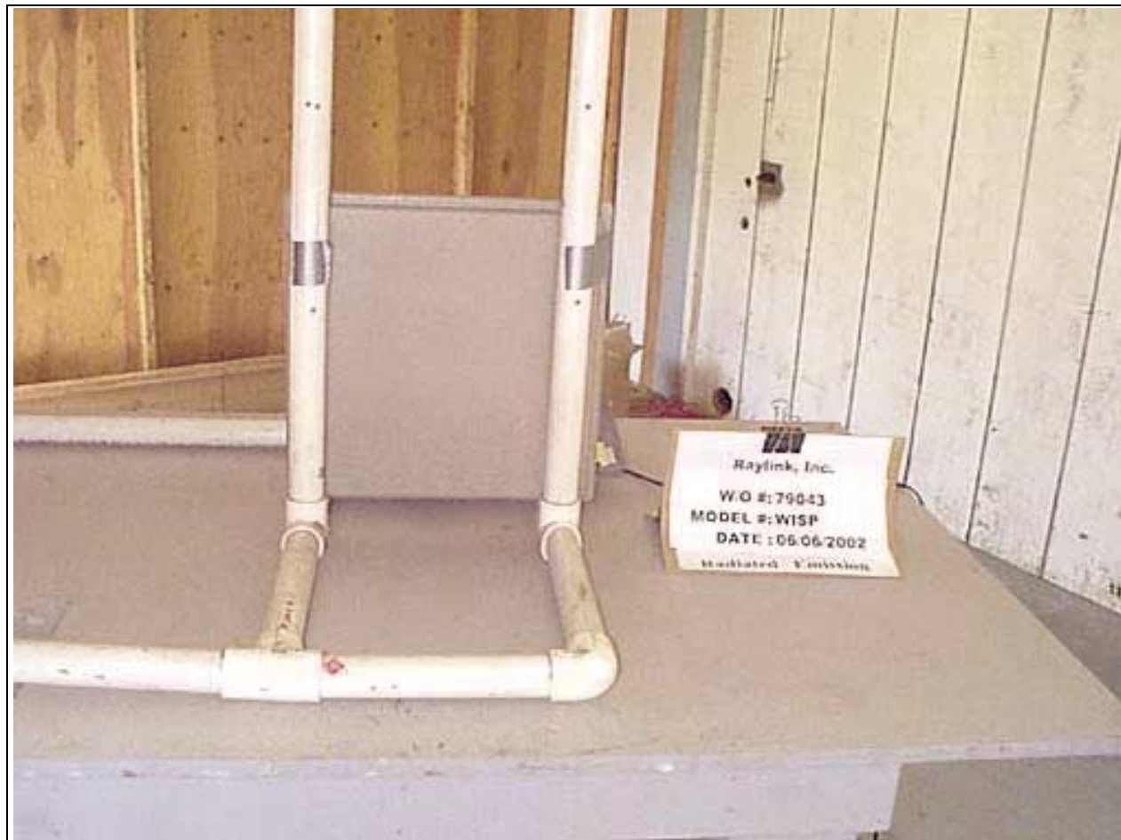
OATS Test Setup - Back View - Biconilog - Mode B
