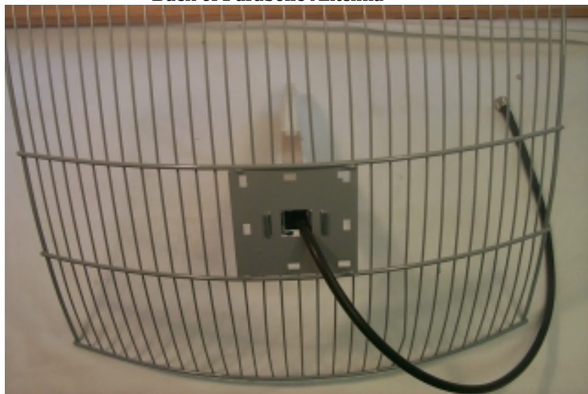
Back of Parabolic Antenna
