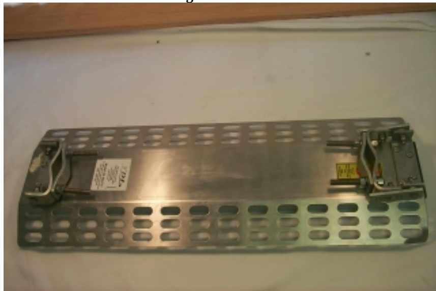
Back of Long Panel Antenna
